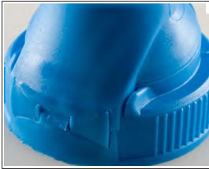
Fig. 28: Web folded inward, flexible hinge
