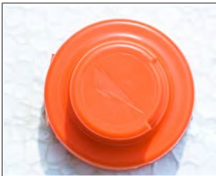
Fig. 32: Circumferential overhang of cap over tooth root
