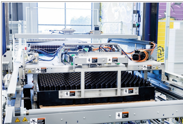
Fig. 1: Fully automatic sweep-off depalletiser with containers in nested container formation
