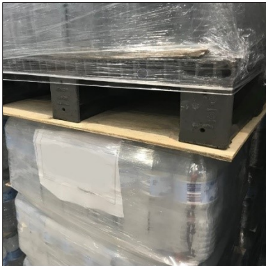
Fig. 55: New container stack with load distribution plate
