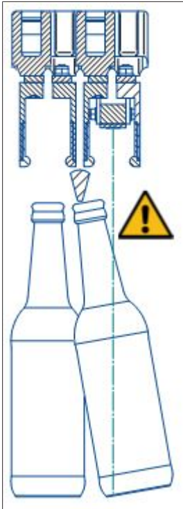
Fig. 5: Collision - The tilted position of a bottle prevents the retraction of the space pre-centring unit
