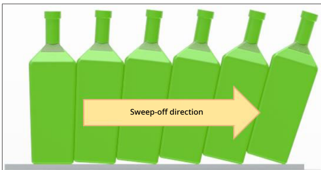
Fig. 73: Tilting problems when sweeping off conical containers
