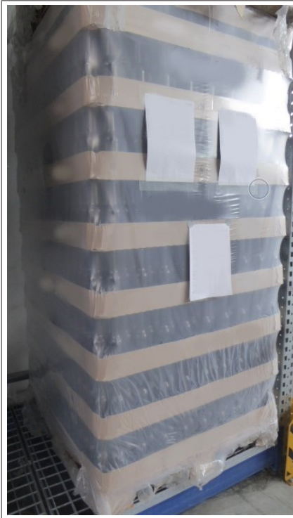
Fig. 7: Optimally aligned new container stack with bottom trays
