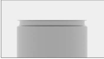
Fig. 81: Side view of a can with still unseamed crimping rim
