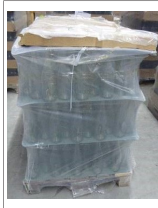
Fig. 11: Stack of new containers with slightly offset inverted trays (manual removal required) and bent-down layer pads
