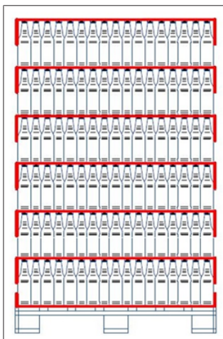
Fig. 51: Inverted tray system with a bottom tray as bottom pad; functionally good for lift-off depalletisers
