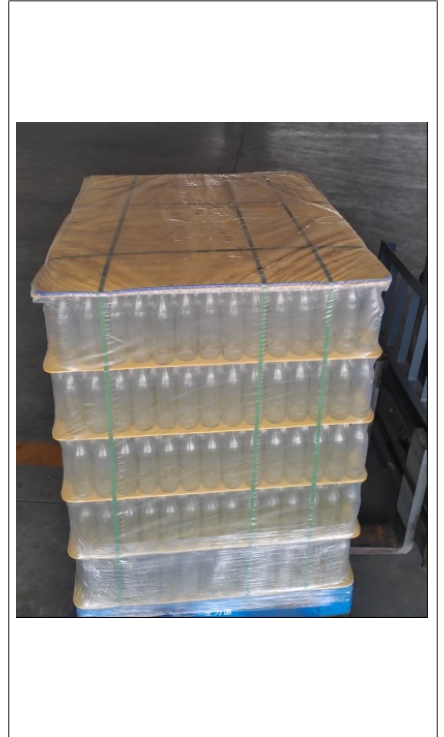
Fig. 8: Optimally aligned new container stack with strapping bands
