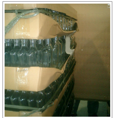
Fig. 19: New container stack with severely deformed bottom trays and slipped containers
