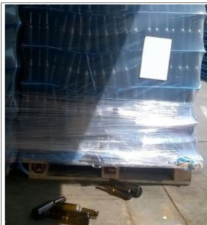
Fig. 17: New container stack with fallen containers
