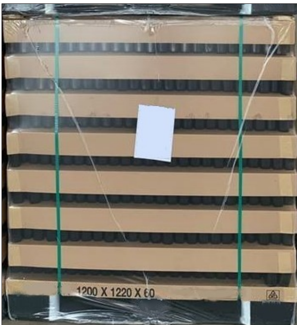
Fig. 56: Green strapping bands with top frame on a new glass stack
