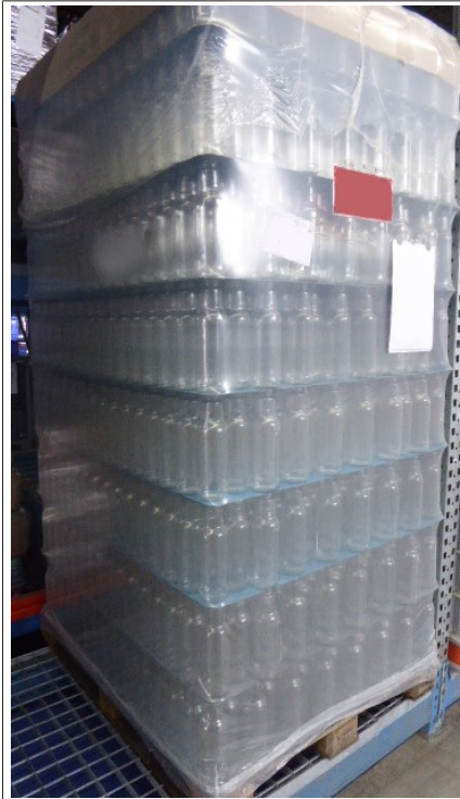
Fig. 6: Optimally aligned new container stack with plastic layer pads
