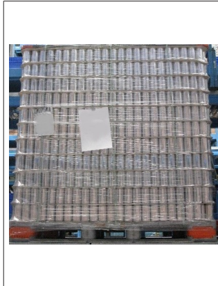
Fig. 10: Stack of new cans with slightly bent-down layer pads in the edge area
