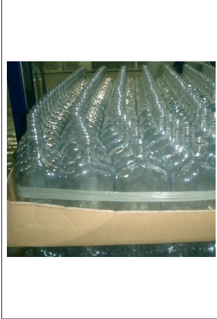
Fig. 13: New container stack with slipped container rows
