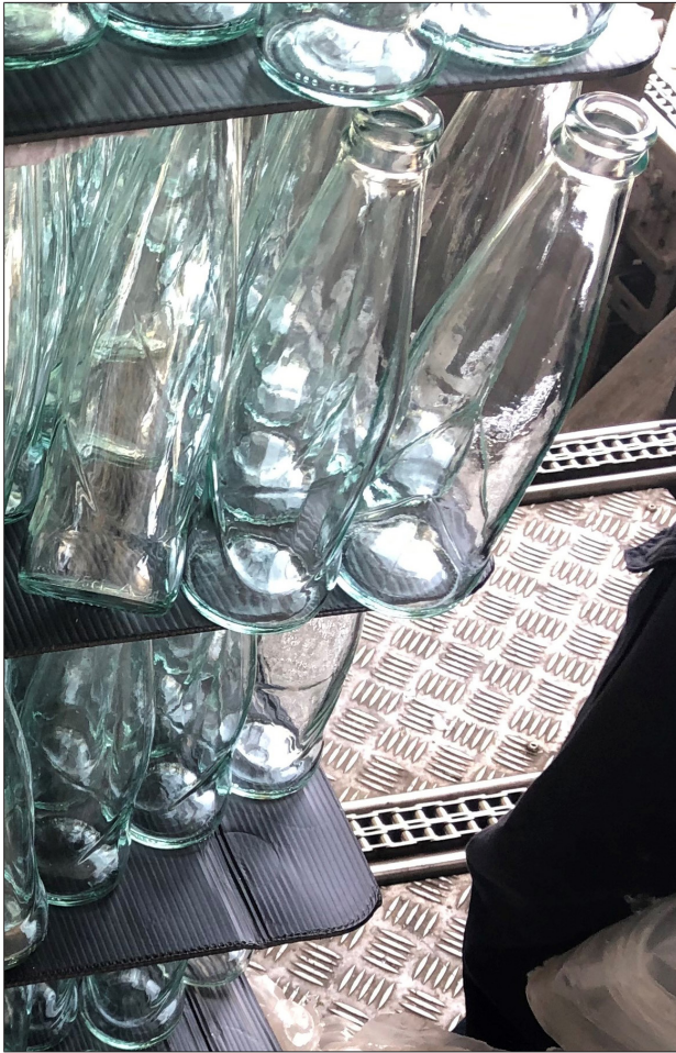
Fig. 44: Corner containers that have fallen down after film removal
