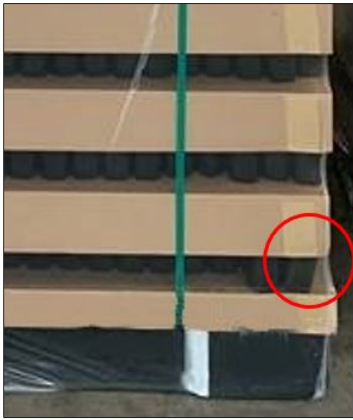
Fig. 53: Stack of new glass containers with inverted trays that are too large and shifted bottles
