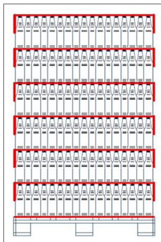
Fig. 50: Inverted tray system with flat bottom pad; functionally good for sweep-off depalletisers
