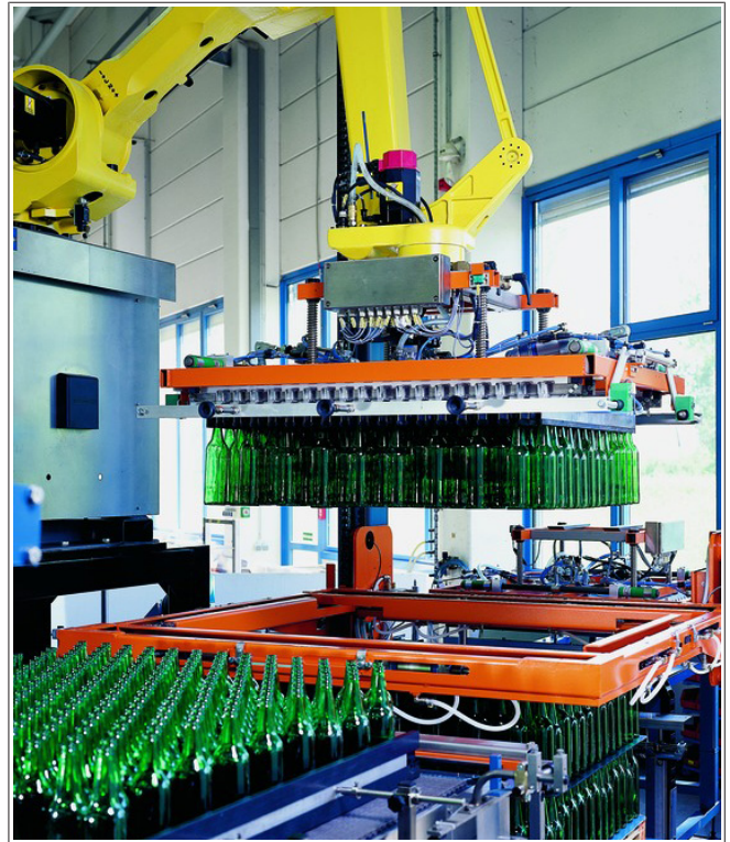
Fig. 4: Fully automatic lift-off with bar or inflated-bar grippers
