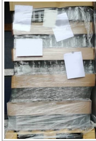
Fig. 15: New container stack with greatly slipped container layers
