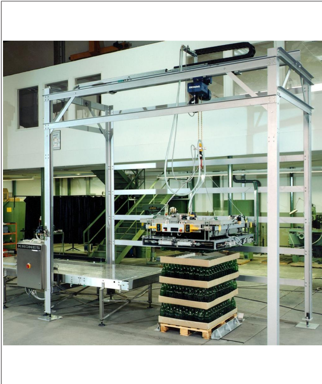
Fig. 3: Semi-automatic gantry lift-off depalletiser with manually controlled bar gripper
