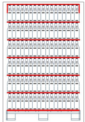
Fig. 52: Layer pad system with no or only one inverted tray as top layer; functionally good for sweep-off depalletisers
