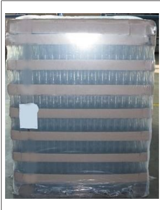
Fig. 9: New container stack with pressed-in inverted tray corners
