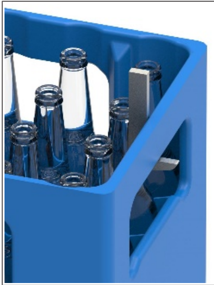
Fig. 25: Hook access in beverage crate (perspective view)
