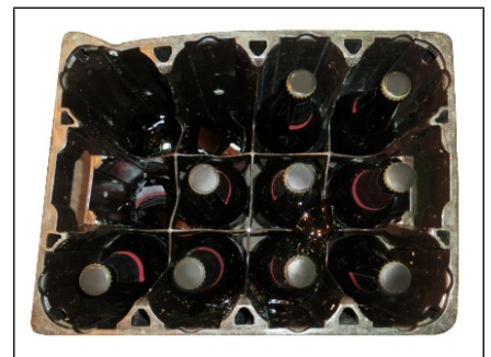
Fig. 45: Pressed-in crate wall
