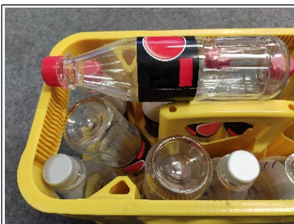
Fig. 43: Damaged and incorrectly oriented PET bottles
