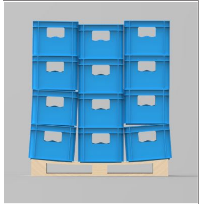
Fig. 73: Pallet lowered downward: Conditionally critical as long as the crates still lock
