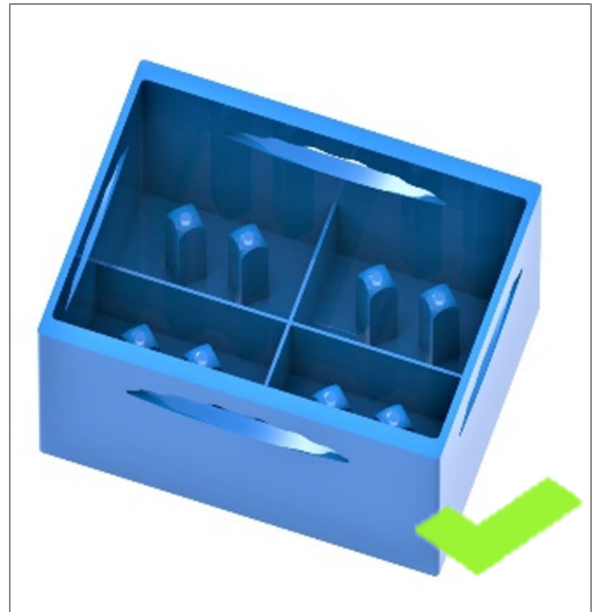
Fig. 82: Pin-partitioned crate without divider bars for individual containers
