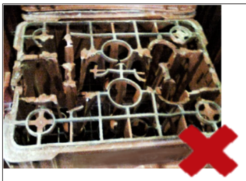
Fig. 67: Broken-out beverage crate base
