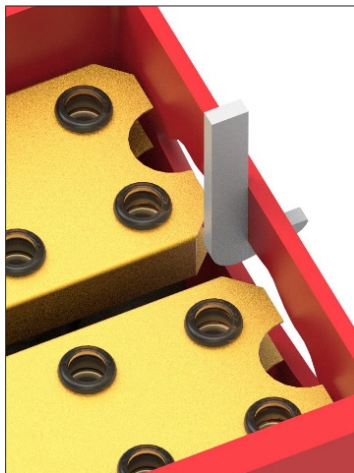
Fig. 80: Beverage crate with multipacks and swivelled-in gripping hook
