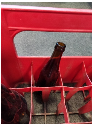
Fig. 59: Glass bottle not completely standing on crate base
