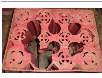
Fig. 44: Chipped crate base
