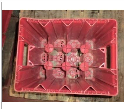
Fig. 42: Slightly pressed-in crate wall
