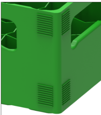
Fig. 32: Horizontal ribs on corner area
