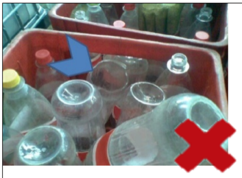
Fig. 68: Beverage crate with incorrectly oriented containers
