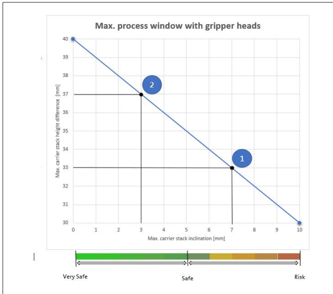
Fig. 139: Areas of permitted stacking height difference depending on tilt
